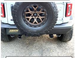
7 After your vehicle has gone through a few heat cycles re torque all your clamps and double check fitment. Use soap and water to clean your black ceramic coated stainless steel tips.
