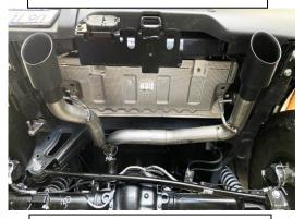
6. Install the tips. They were designed to have a .75" of an inch clearance from the bumper. Adjust pipes and all connections to find that perfect fit. Begin to tighten all connections from the front to the back. Double check you tip exit locations after each connection is tight.
