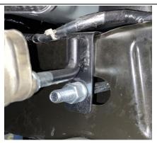
4. Install the rear supplied Hanger brackets to the factory frame rail. There will be large existing holes in the frame for the hangers to be installed to. Keep loose until everything is installed
